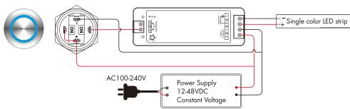
Connect with self-resetting metal button, positive trigger input.
