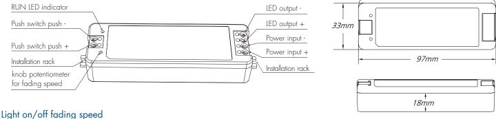
Rotate knob to switch fading speed, when the fading speed set to 1/3/5/10/20s, the RUN LED indicator will flash 1/2/3/4/5 times.
