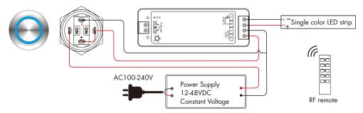
• Connect with push switch panel, negative trigger input. Press the panel to switch or adjust brightness.
